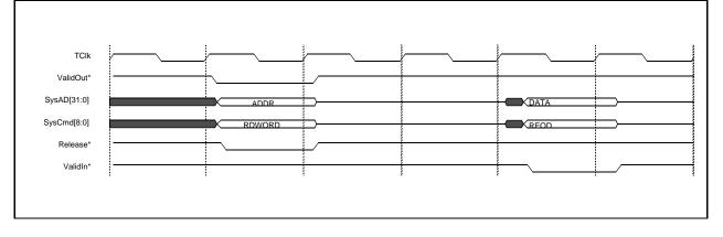
Figure 2: Single Word Read Through CPU/Local Master Interface
