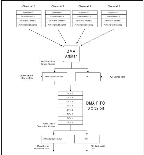
Figure 24: DMA Controller
