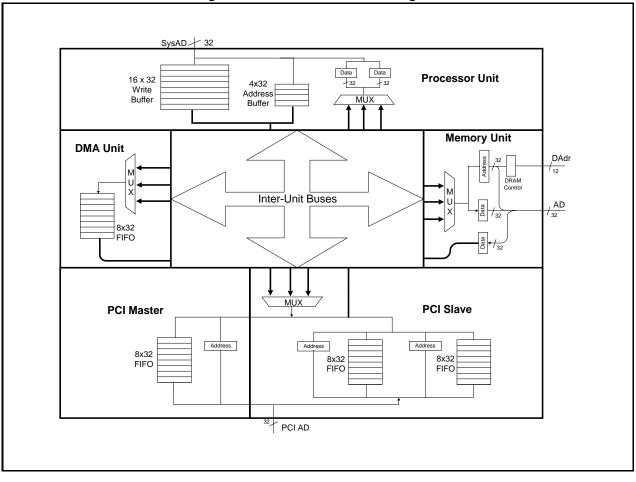
Figure 1: GT-64111 Internal Block Diagram
