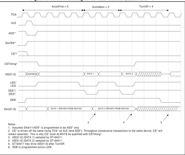
Figure 17: Waveform Showing Device Read Parameters, LatchFunct = 1
