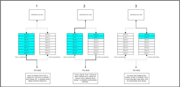
Figure 23: PCI Target Interface FIFOs Operational Example
