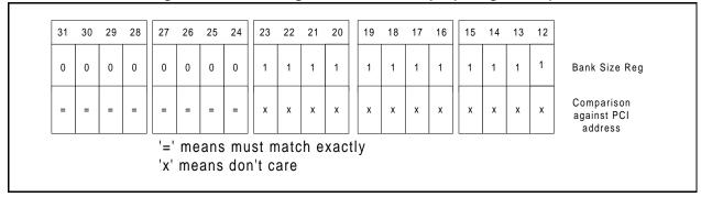
Figure 8: Bank Size Register Function Example (16Meg Decode)
